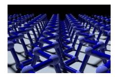
Two-dimensional phosphane, a material known as phosphorene, has potential application as a material for semiconducting transistors in ever faster and more powerful computers. But there's a hitch. Many of the useful properties of this material, like its ability to conduct electrons, are anisotropic, meaning they vary depending on the orientation of the crystal. Now, a team including researchers at Rensselaer has developed a new method to quickly and accurately determine that orientation using the
