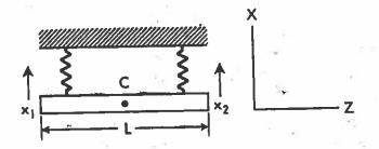
The springs have the same force constant k. The motion of the center of gravity is constrained to move parallel to the vertical x-axis. Find the normal modes and frequencies of vibration of the system, if the motion is constrained to the xz-plane.
